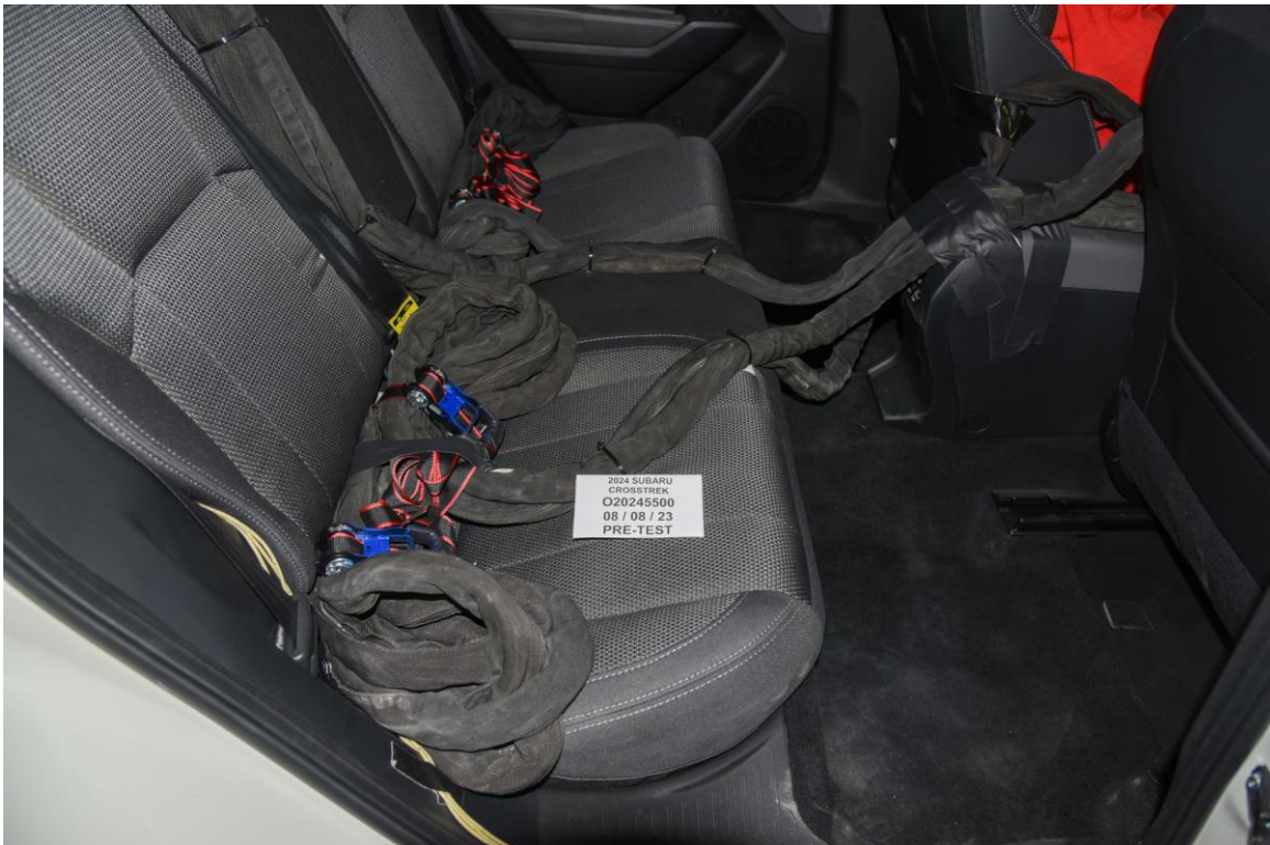
FIGURE 28. Pre-Test Dummy Cable Routing
