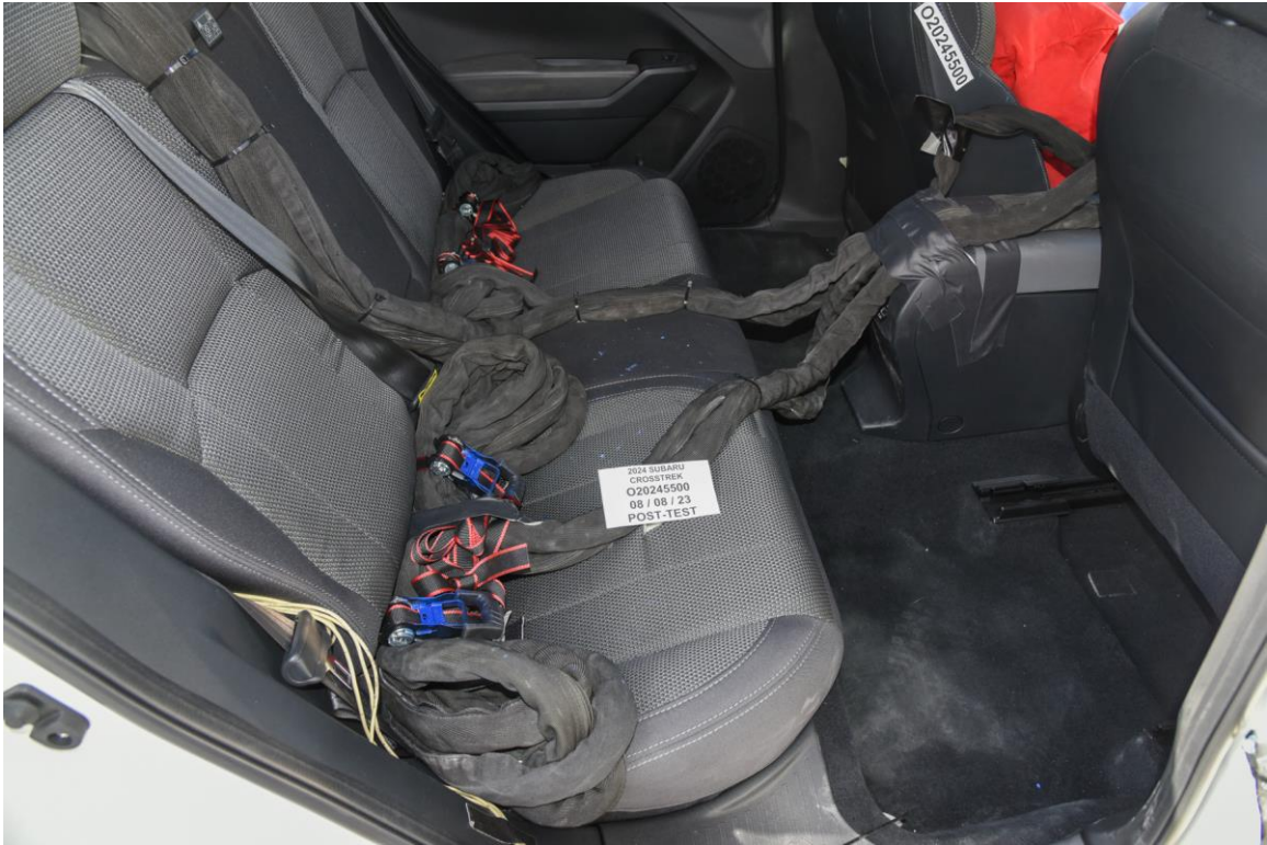
FIGURE 29. Post-Test Dummy Cable Routing
