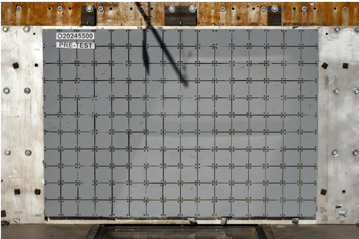
FIGURE 2. Pre-Test Load Cell Wall
