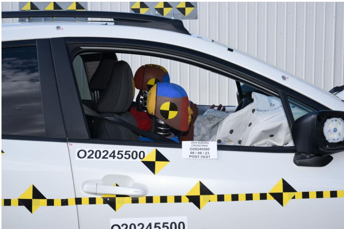
FIGURE 56. Post-Test Passenger Dummy Window View
